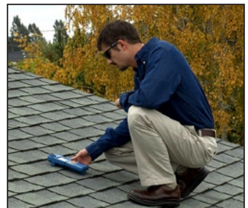
Measuring roof pitch is now integrated into the SunEye 210. Simply lay it on the roof or module and read tilt and heading.
