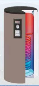
Tank - Steel 6837, DIN EN 10120, P245NB - Double Enameling 1580 degrees - Supplied with a Mg anode. Anti-corrosive protection Flange for easy interior cleaning - Serpentine Coil - Steel plate ST 37.2 Coating. Enamel (vitrified steel) - Insulation CFC free (105-211 gal.) Polyurethane density: 40 kg/m3 - Thickness: 2" Insulation foam (211-264 gal.) - Working pressure 116 psi Maximum 174 psi Maximum temperature 185° F
